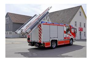
The free space required for roof access can now be used for equipment. Since the shutters are also rolled up on the roof, this means optimum use of space. Besides, no additional personnel is needed, and the pre-coupled suction hoses save additional time. The system is controlled via a Z-Control handheld of the latest generation.
