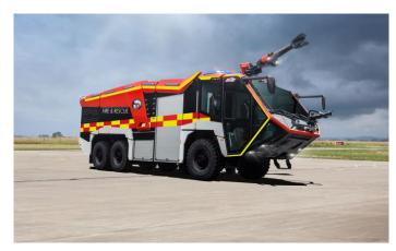
The Crashtender will be built on a TITAN 6x6 chassis with steering rear axle and is equipped with a Scania 770 HP V8 engine. Furthermore, the vehicle will be equipped with a 12,000 I water tank, a 1,500 I foam tank and 250 kg extinguishing powder. The Z-Cab AiR is certified according ECE R 29-3 and therefore guarantees highest occupant protection. The vehicle will be controlled and operated via Z-Control of the latest generation according to the whole ZIEGLER line
