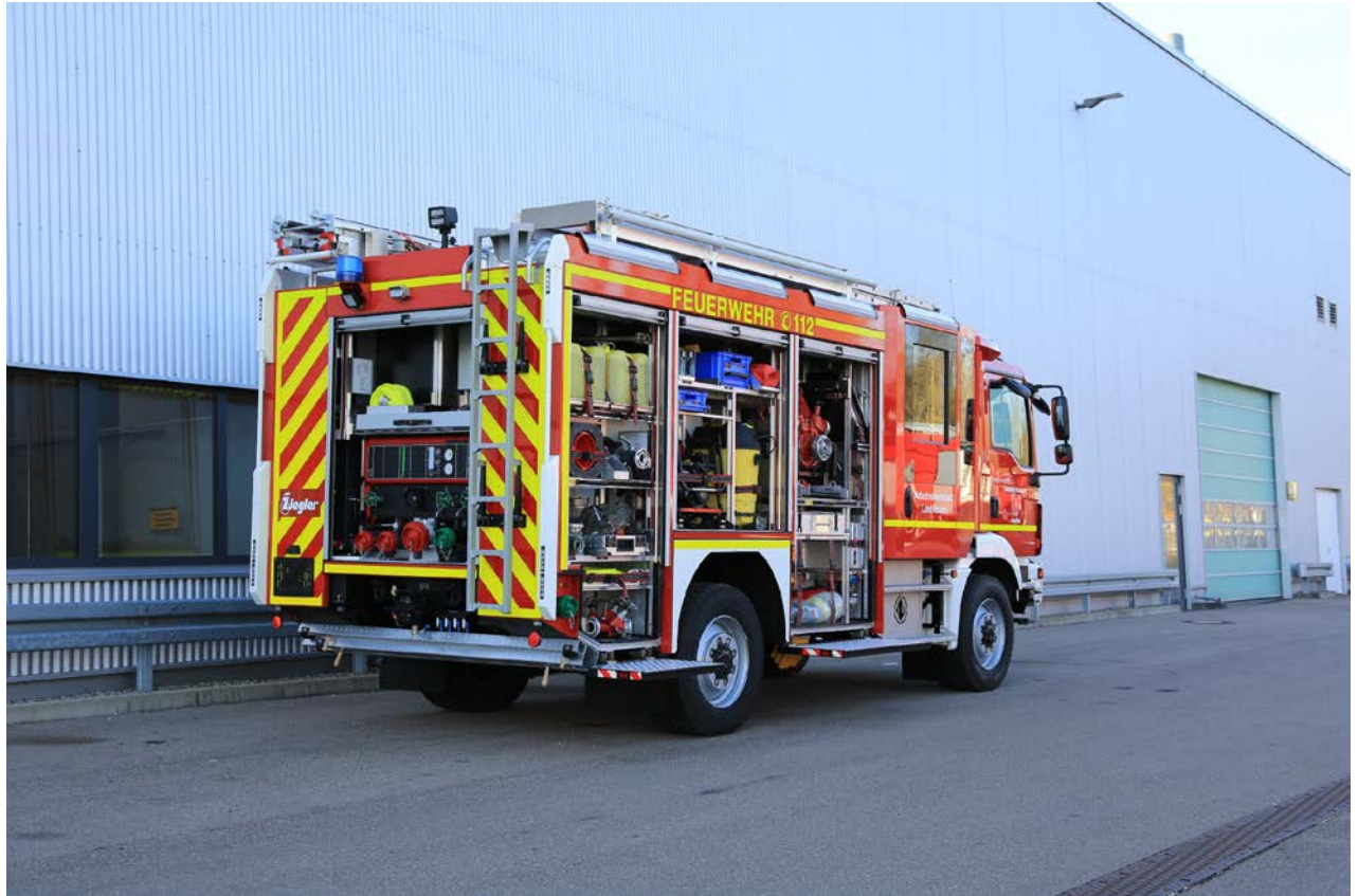
First LF 10 KatS vehicle from the 10th Hesse state procurement campaign on a MAN TGM 13,250 4x4 Euro 6 chassis
