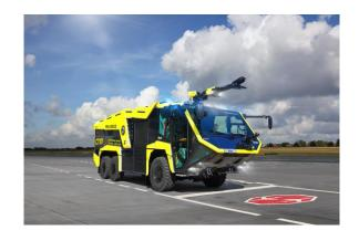
ZT-6000 as a roof mounted turret), the rapid intervention unit and the self-protection system with extinguishing power. The Z-Cab Air is certified according ECE R 29-3 and therefore guarantees highest occupant protection. The vehicle will be controlled and operated via Z-Control of the latest generation according to the whole ZIEGLER line.
