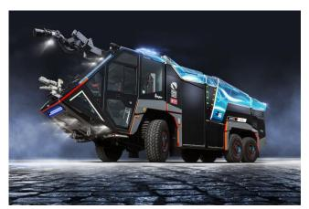
The Z6 HYBRIDDrive by ZIEGLER is a 6x6 ARFF which can drive in three modes. Pure electrical mode; combined electric and combustion mode; and purely with a conventional, low emission engine.
