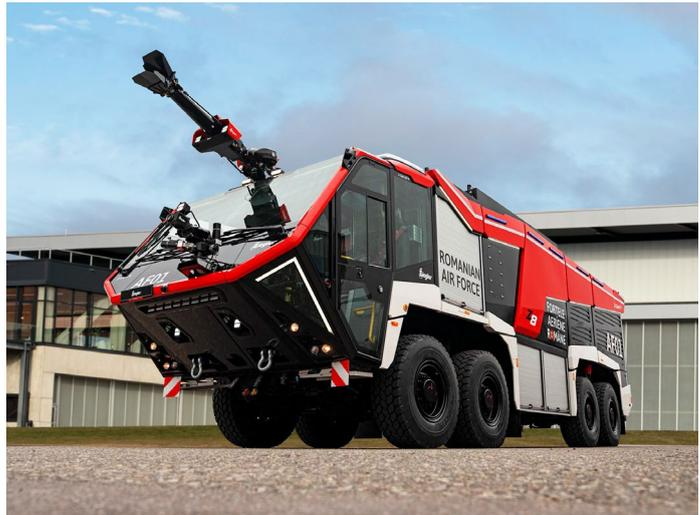
Equipped with two powerful traction motors, the vehicle reaches a top speed of 140 km/h and offers excellent acceleration values, even under demanding climatic and geographical conditions. The proven ZIEGLER extinguishing technology ensures maximum efficiency in operations where every second counts.
